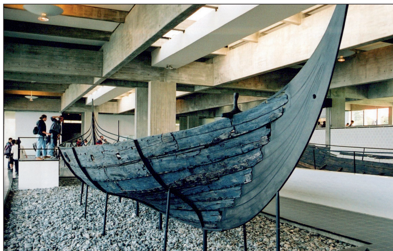
ABOVE: An early clinker-built Viking ship. The design proved to be very significant for better seafaring in the middle ages.
