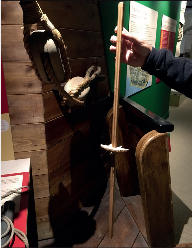
ABOVE LEFT: The cross-staff was a graduated stick having a sliding vane. It was used to measure the elevation of stars, but only in later medieval times, it appears.
