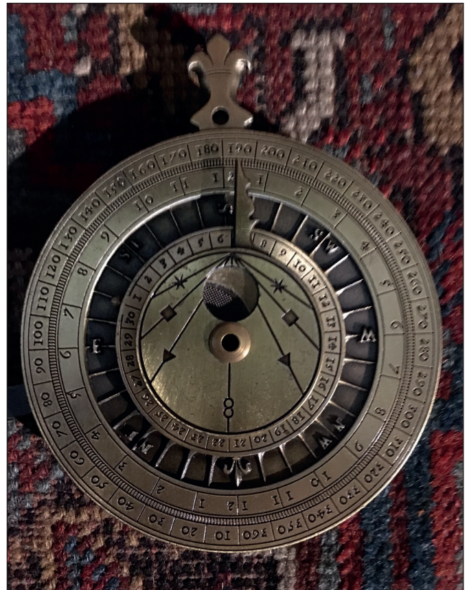
ABOVE LEFT: A Traverse Board was used for keeping track of a course steered during watches. ABOVE RIGHT: A Tide Computer - a device for calculating the height of the tide. BELOW: Two Night-Time Clocks.
